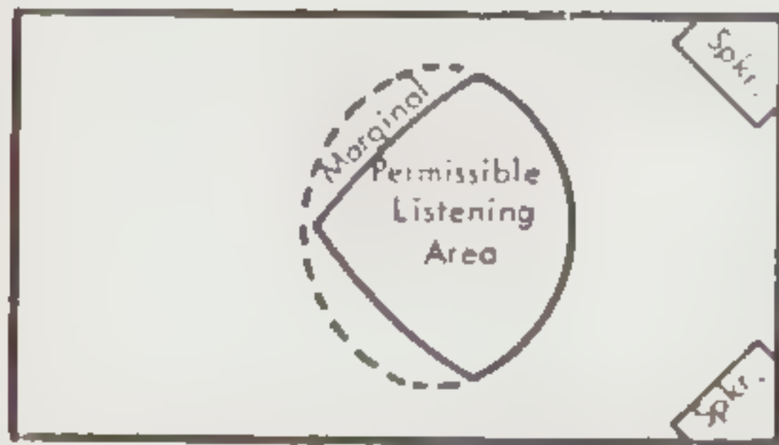
Fig. 1. Permissible listening area denotes the area where satisfactory stereophonic listening occurs with speakers in natural corners on the short wall of a room of 2:3 width to length ratio. The area is less than one-fourth the area of the room.
